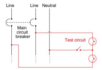
The electrician tells you to open and close the switch, and observe the brightness of the light bulbs. This will indicate whether or not the system is 3-phase.
