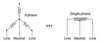
An experienced electrician suggests you build the following circuit to test whether or not the home's power is supplied by a 3-phase source or a single-phase source:
